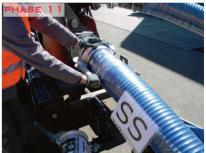
**PHASE 11**: A ballasting operator supports the hose while the second Ballasting Operator release the main quick coupling.
