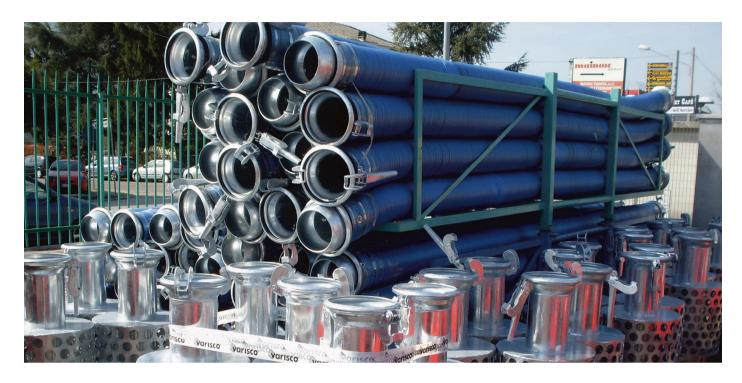
The pipe lines of the system are composed by hoses with a diameter of 8" equivalent to 200mm. This size allows the reduction and optimization of the loss of pressure during pumping. In case of emergency the pump flow can require to be reversed. Fagioli always arrange contingency hoses close to the pumps in order to be quickly connected to the pumps reversing the flow if required.
