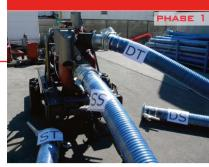
PHASE 1: Switch-off the engine pump.
